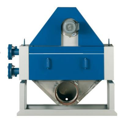
The condensing heat exchanger can be provided with a separately mounted starter control box and a water flow switch. The **control box** incorporates connections for a three phase supply, the centrifugal fan motor, the water flow switch, boiler/burner operation contacts and fan motor lock out
